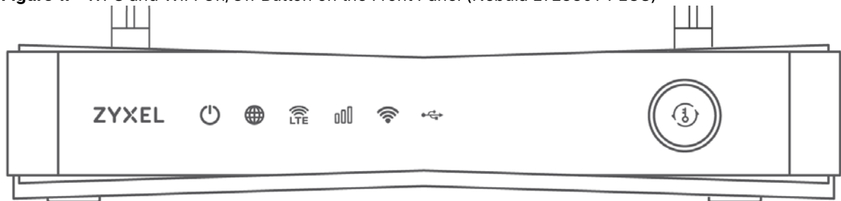
Figure 17 WPS and WiFi On/Off Button on the Front Panel (Nebula LTE3301-PLUS)
