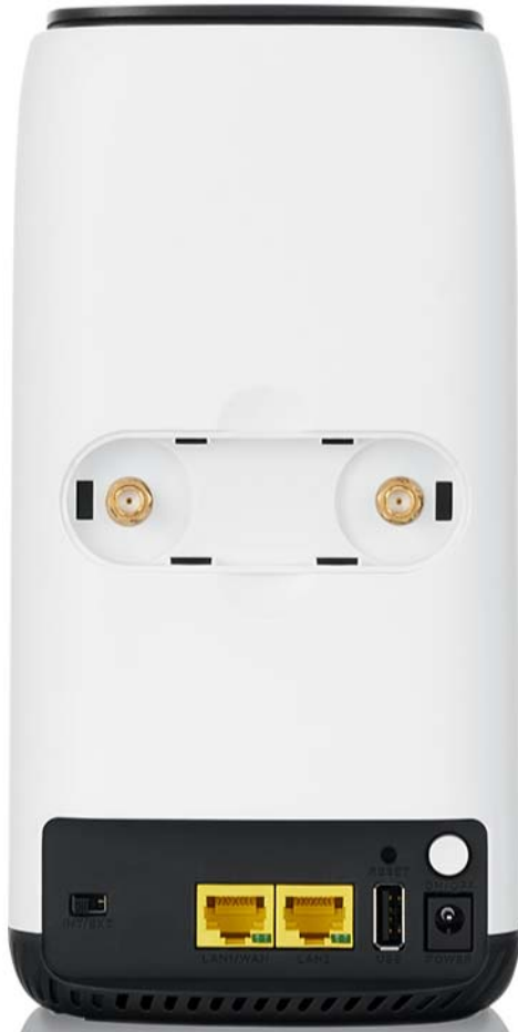
Figure 20 Antenna Ports on the Rear Panel (NR5101)
