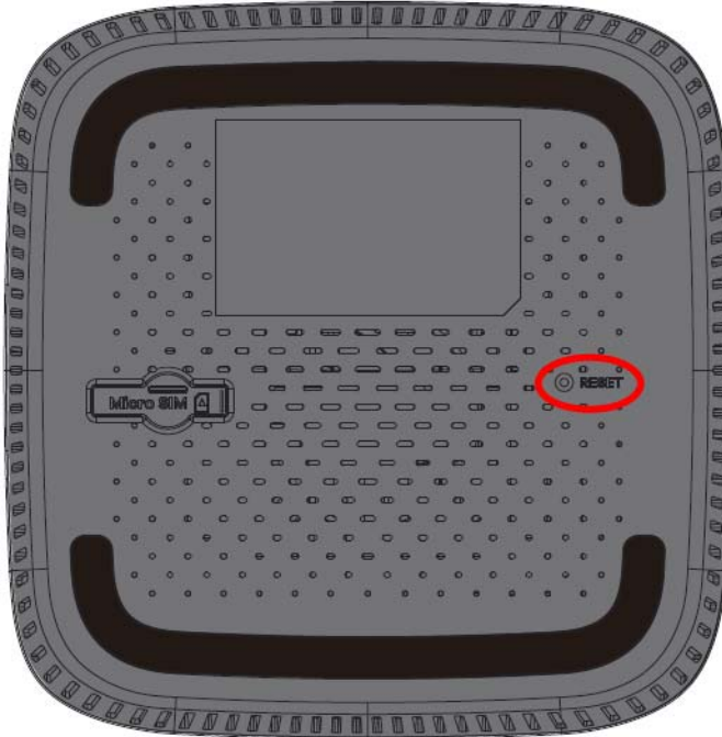
Figure 29 Micro SIM card slot and RESET button on the bottom panel (Nebula FWA510)
